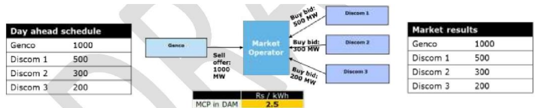
Chart 7: Overall scenario of quantum self-scheduled by discoms, bidding and market clearing for a particular 15-min time block in case the generator participates in MBED and sell 1000MW through DAM
